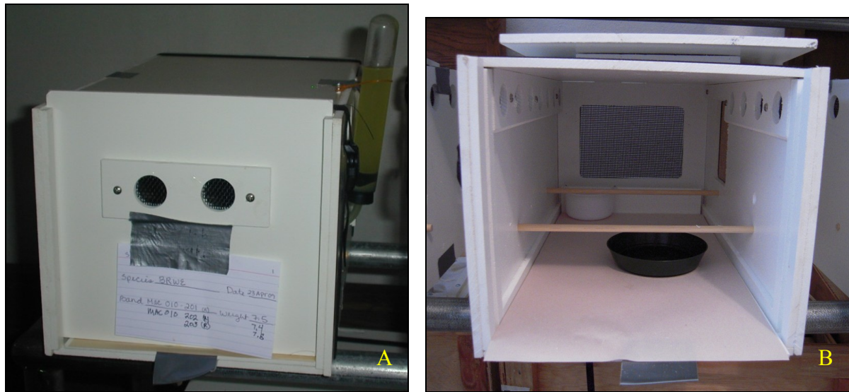
Figure 2. Details of the Bridled White-eye holding containers used on Tinian, April 2009: A) front closed with nectar container attached; B) front open, detailing the perches, back ventilation opening, and 3 mm thick Sintra PVC false floor.
