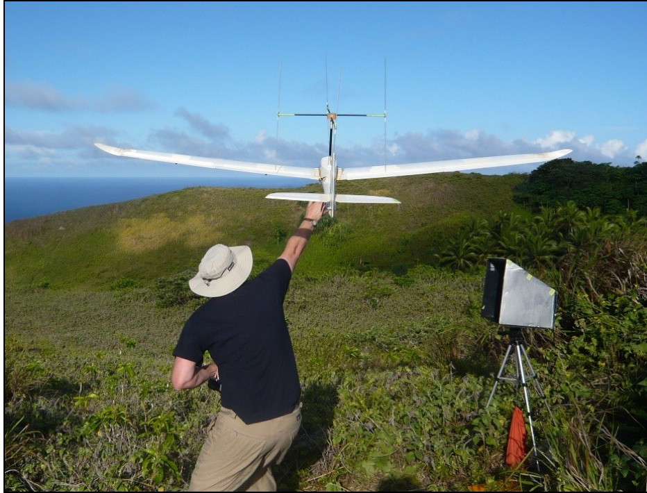
J. Burt launching aircraft with radio tracking pod attached. The ground station laptop computer is housed in the shade box to the right.
