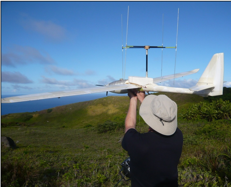
Figure 1. Cularis sailplane (UAV) with mounted radio tracking (RT) pod as test flown on Sarigan, May 2009.
