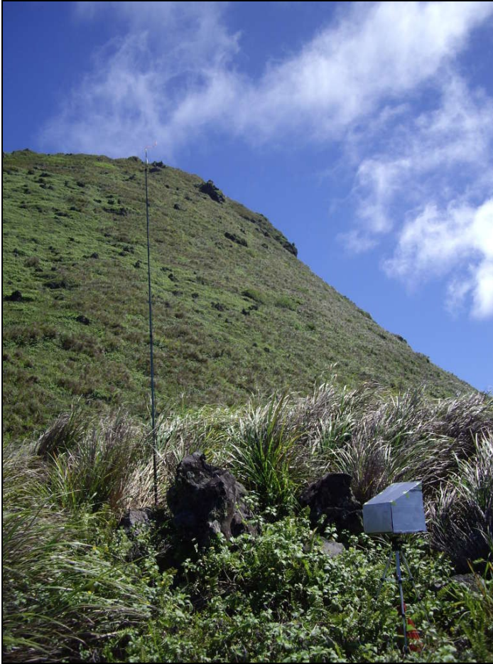
Figure 2. Ground station setup with radio modem antenna and laptop computer shade-box, Sarigan, May 2009.
