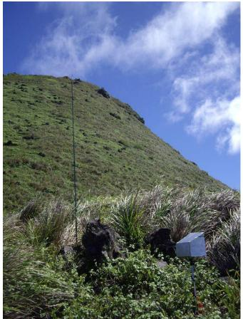
Figure 2. Ground station, radio modem antenna mast and laptop shade box were located on a small hill at the NE corner of the plateau, about 70m from the campsite.
