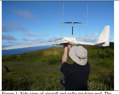
Figure 1: Side view of aircraft and radio tracking pod. The four vertical antennas are used by the system to detect radio tag transmissions and generate an angle to the signal source relative to the nose of the plane. Multiple tag pulse detections at different aircraft locations allow the signal source to be triangulated.
